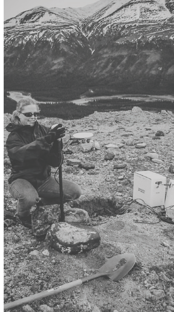
GI-UAF graduate student Kelly Kore installing a temporary seismic station to monitor aftershocks from Denali fault earthquake.
